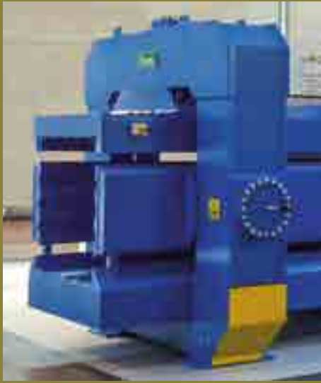
Portale strettoio (3 cilindri). Counter pressure device with gantry.
